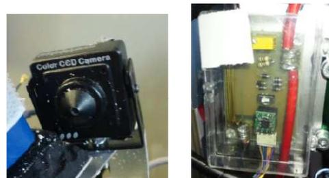
(a) CCD camera (b) Wattmeter
