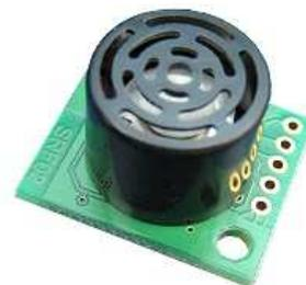
The SRF02 is a single transducer ultrasonic rangefinder . It features both I2C and a Serial interfaces[4].In order to distance measurement we used I2C interface. The proposed method to velocity measurement is calculating the difference between two height in determined
