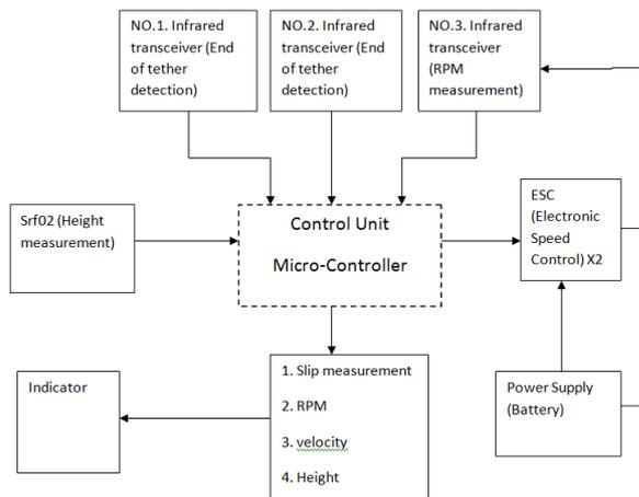
In data measurement part, the tires slip is measured using N.O.3 infrared transceiver and the ultrasonic sensor, SRF02. N.O.3 infrared transceiver measures the motor RPM using a mark on the motor and forms a simple encoder. Using height difference in a determined time, velocity will be measured and the indicator displays the data.
