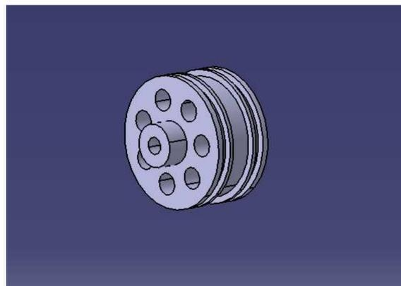
After that, by lathing and milling, we made them .the pulleys and rings material is aluminum. We tried to reduce weight of components by drilling. Control car tires are used as the climber tires.
