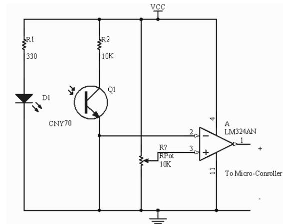
As seen on this figure suitable output for detecting end of tether will be generated by the reflected light from the tether surface to the base lead of transistor Q1. The LM324 output is connected to external interrupts of an atmega32 micro controller. In N.O.1 interrupt routine service the climber will come down and in the other external interrupt routine service the climber will be stopped.
